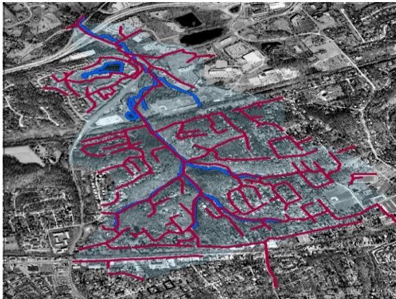
Sewer lines along Crabby Creek- all narrow the streambed and are a sediment supply during high water
